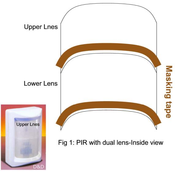
This technique of covering the PIR field view is working in single or dual lens PIR.
