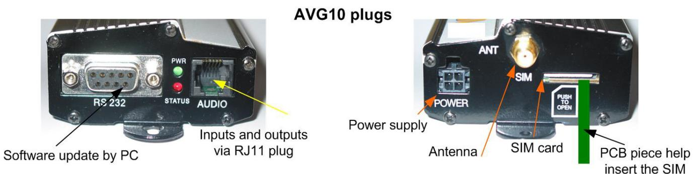
Figure 1: AVG10-G wiring
