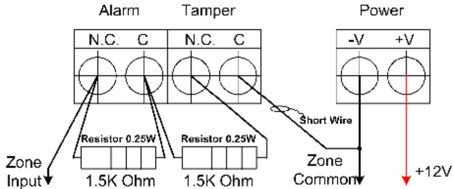
Figure 1A: European Double-Pole wiring drawing
