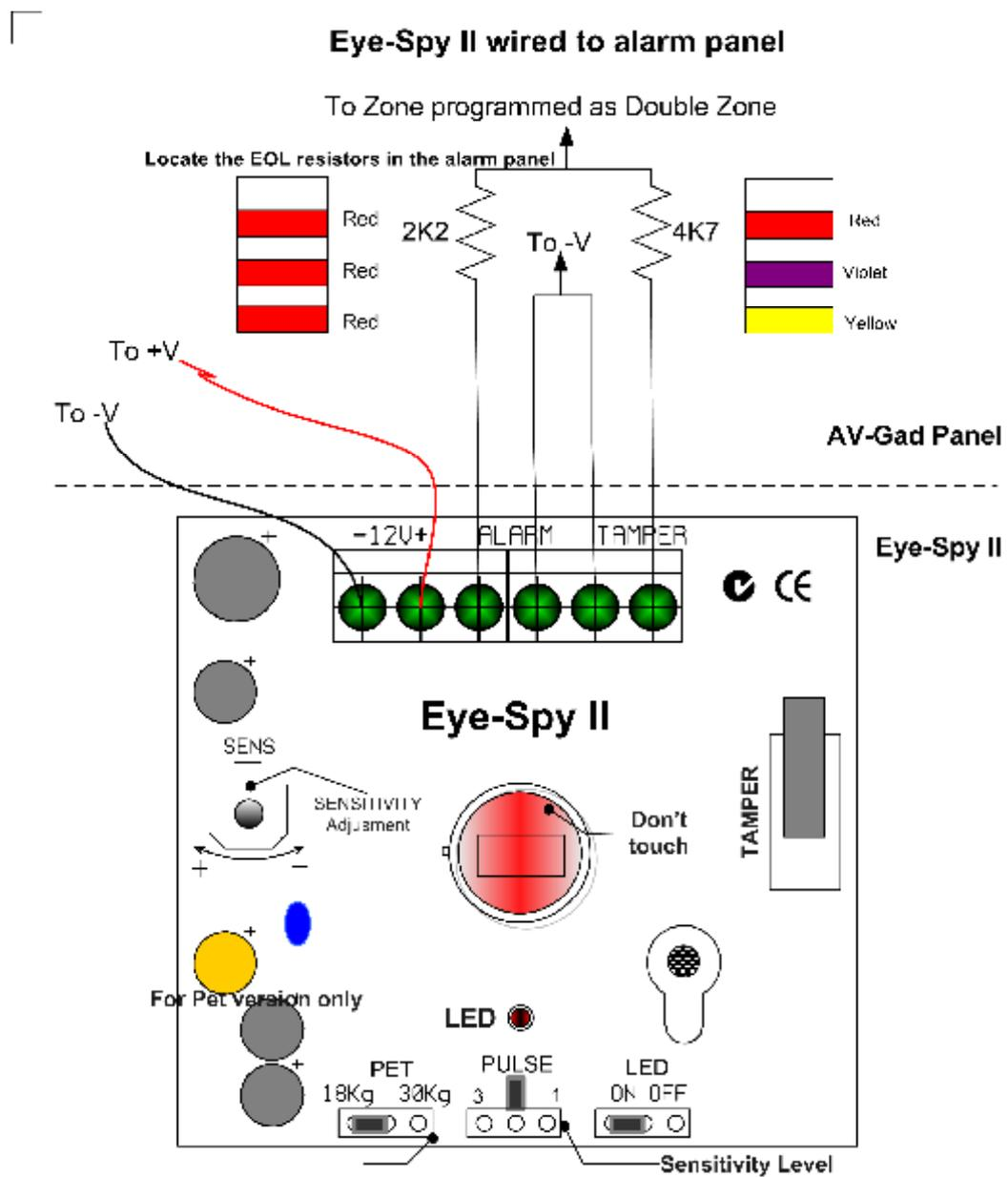
Figure 1: Double-Zone Wiring to Eye Spy II
